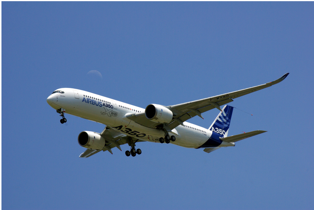
Fig. 1.1. Picture of A350-900 during landing. The nose landing creates wake vortices. They are convected under the fuselage and interact with the main landing gear doors. This induces vibrations leading to structure fatigue or even to rupture.
